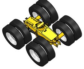
Capacity: 0-5 mph 45 Tons 5-15 mph 40 Tons 15-55 mph 30 Tons
